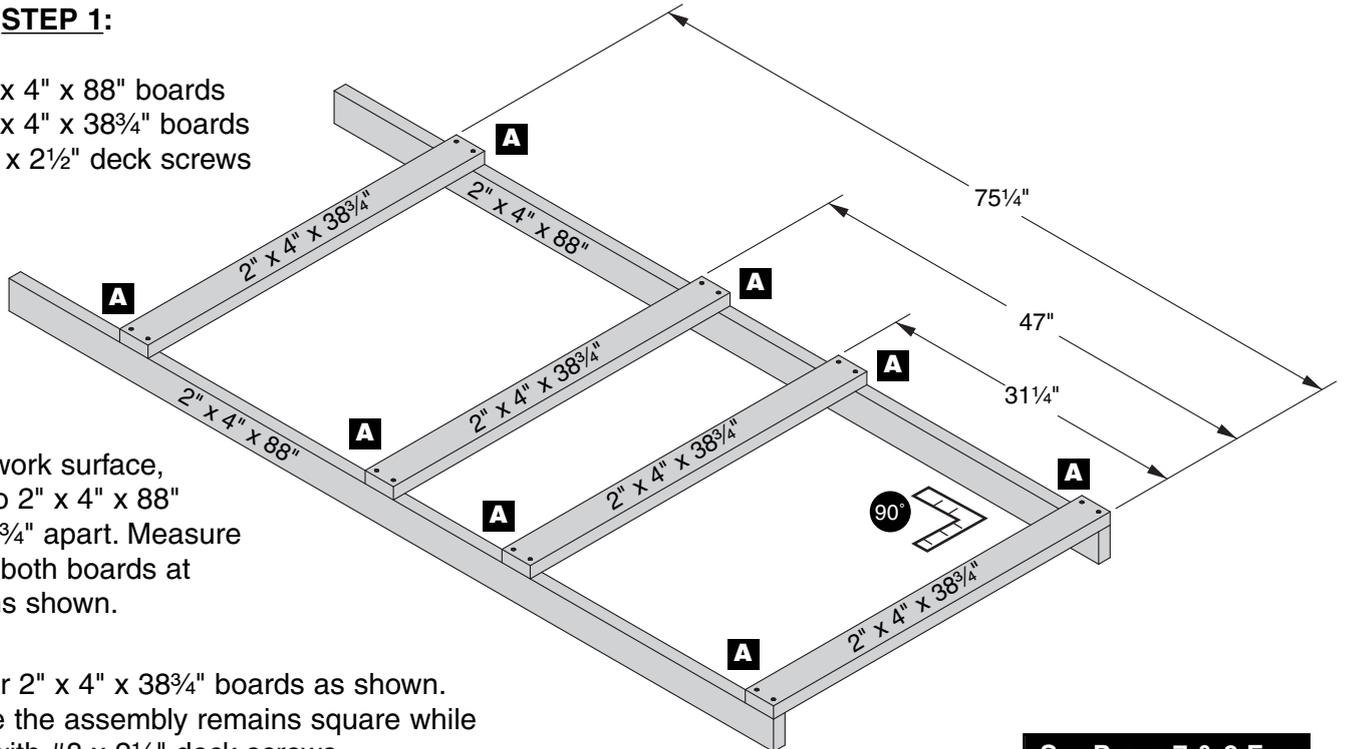
On a flat work surface, lay out two 2" x 4" x 88" boards 38<sup>3</sup>/<sub>4</sub>" apart. Measure and mark both boards at dimensions shown.
