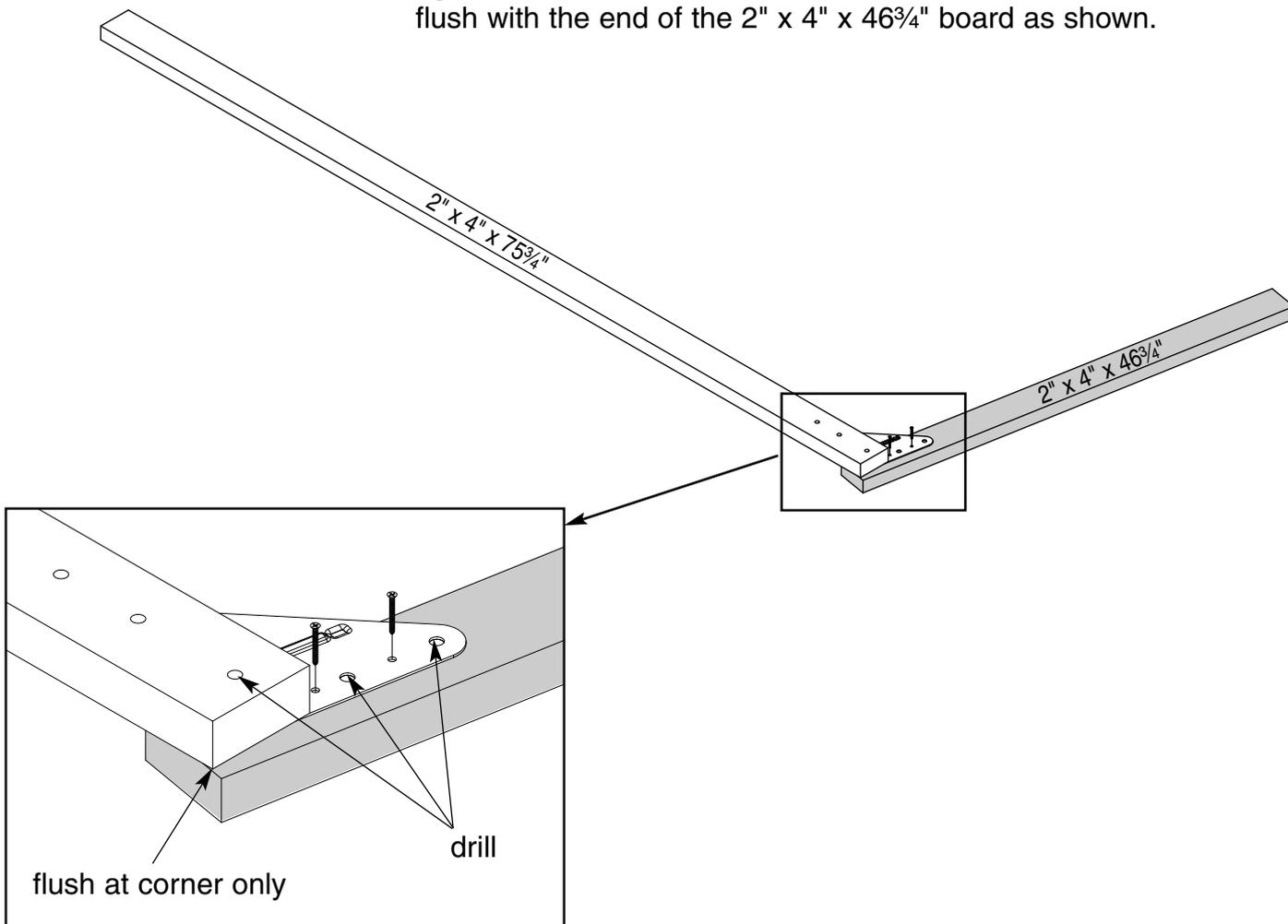
Use the bracket as a drill guide and drill two <sup>1</sup>/<sub>8</sub>" holes 1" deep into the boards. Attach with #8 x 1<sup>1</sup>/<sub>4</sub>" deck screws.
