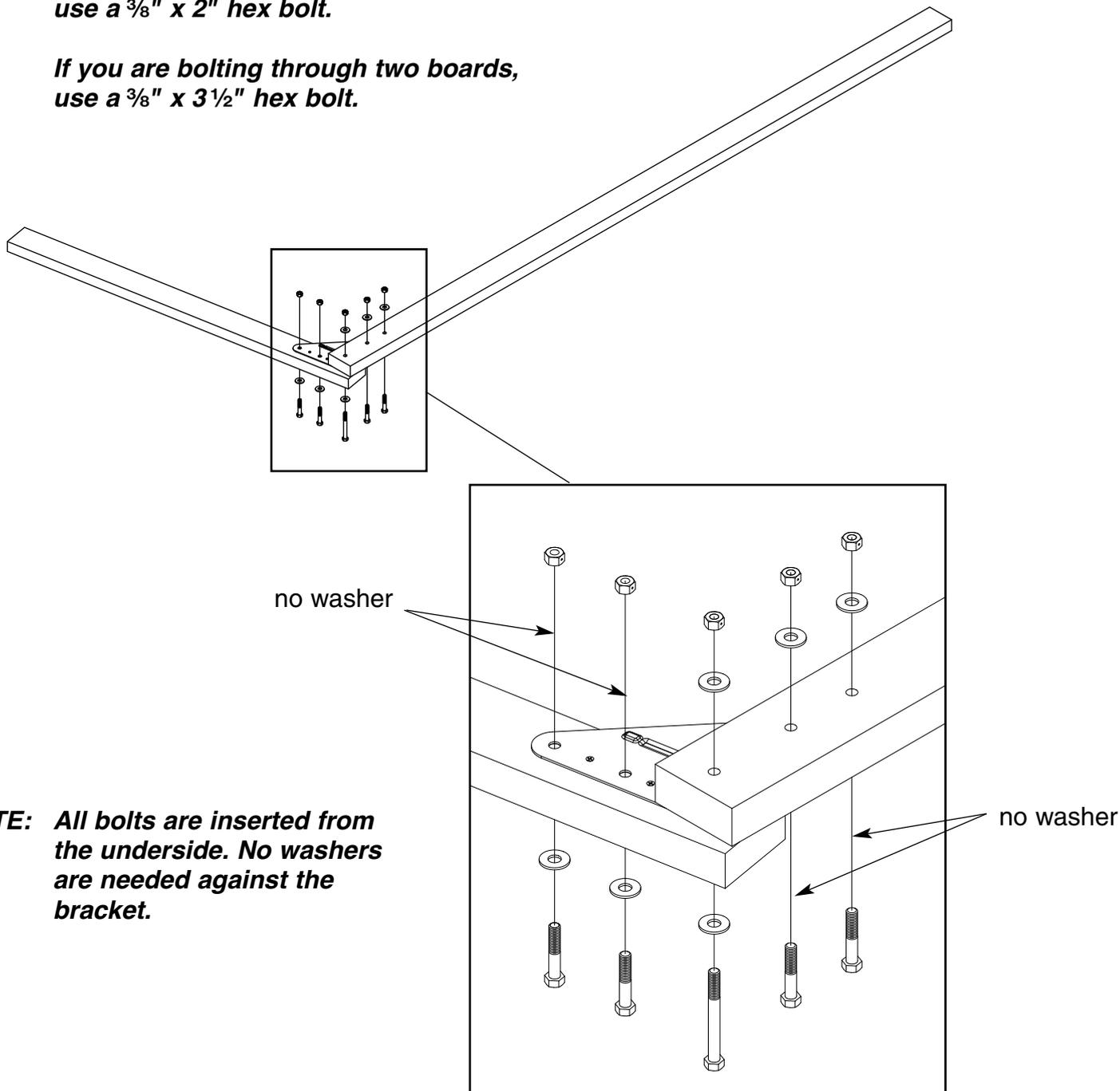
**NOTE:** *All bolts are inserted from the underside. No washers are needed against the bracket.*
