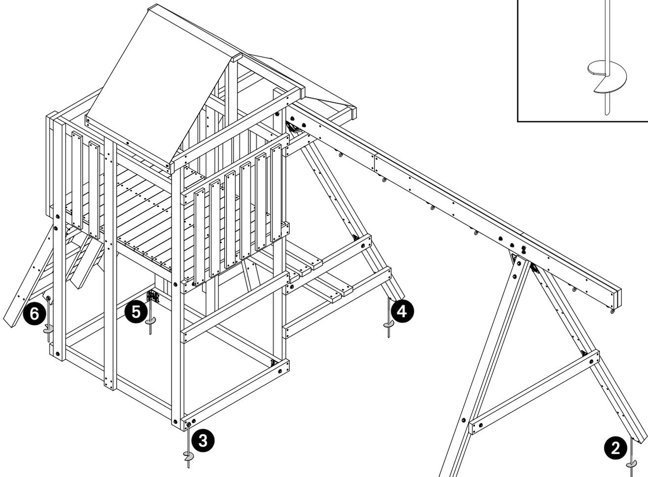
**Note:** If soil conditions permit anchors to be pulled out easily, such as in sandy soil conditions, cementing is required. If your ground is too hard to screw in the anchors you can remove the earth with a shovel. Install the anchors and compact the earth as you replace it. Anchors must be placed below the level of the shock-absorbing surfacing material to prevent tripping or injury resulting from a fall.
