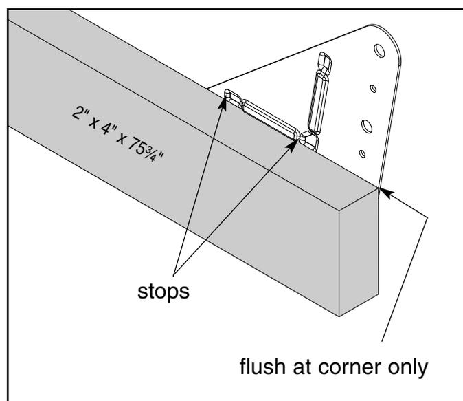
Use the bracket as a drill guide and drill two 1/8" holes 1" deep into the board. Attach with #8 x 1 1/4" deck screws.
