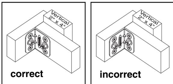
**Caution:** If the bracket was flipped and the short side was against the double board when you drilled, the holes will be too close to the edge of the vertical 2" x 4".
