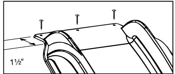
2. Attach slide temporarily to play deck with three #14 x 1¼" screws provided.
