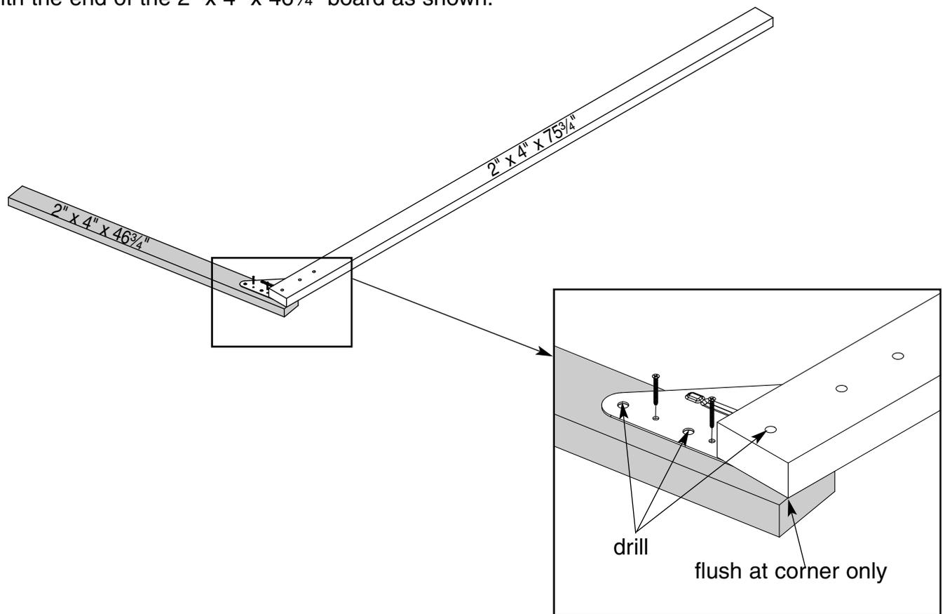
Use the bracket as a drill guide and drill two 1/8" holes 1" deep into the boards. Attach with #8 x 1<sup>1</sup>/<sub>4</sub>" deck screws.
