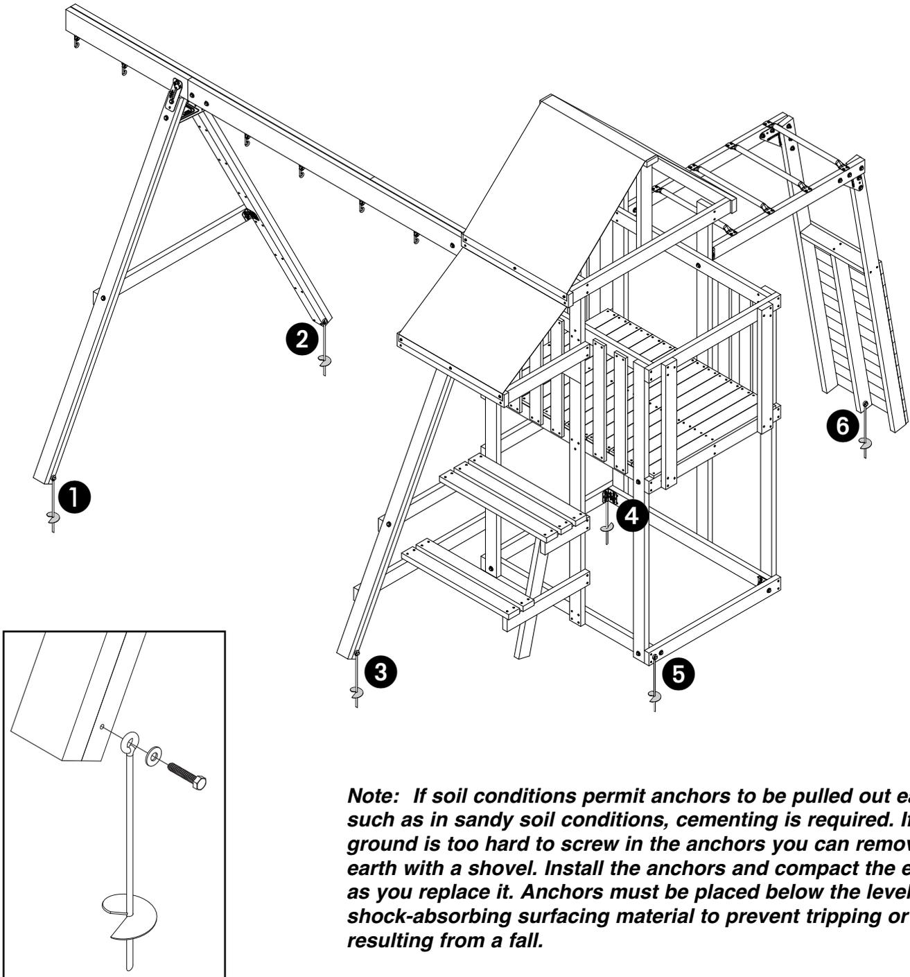
**Note:** If soil conditions permit anchors to be pulled out easily, such as in sandy soil conditions, cementing is required. If your ground is too hard to screw in the anchors you can remove the earth with a shovel. Install the anchors and compact the earth as you replace it. Anchors must be placed below the level of the shock-absorbing surfacing material to prevent tripping or injury resulting from a fall.
