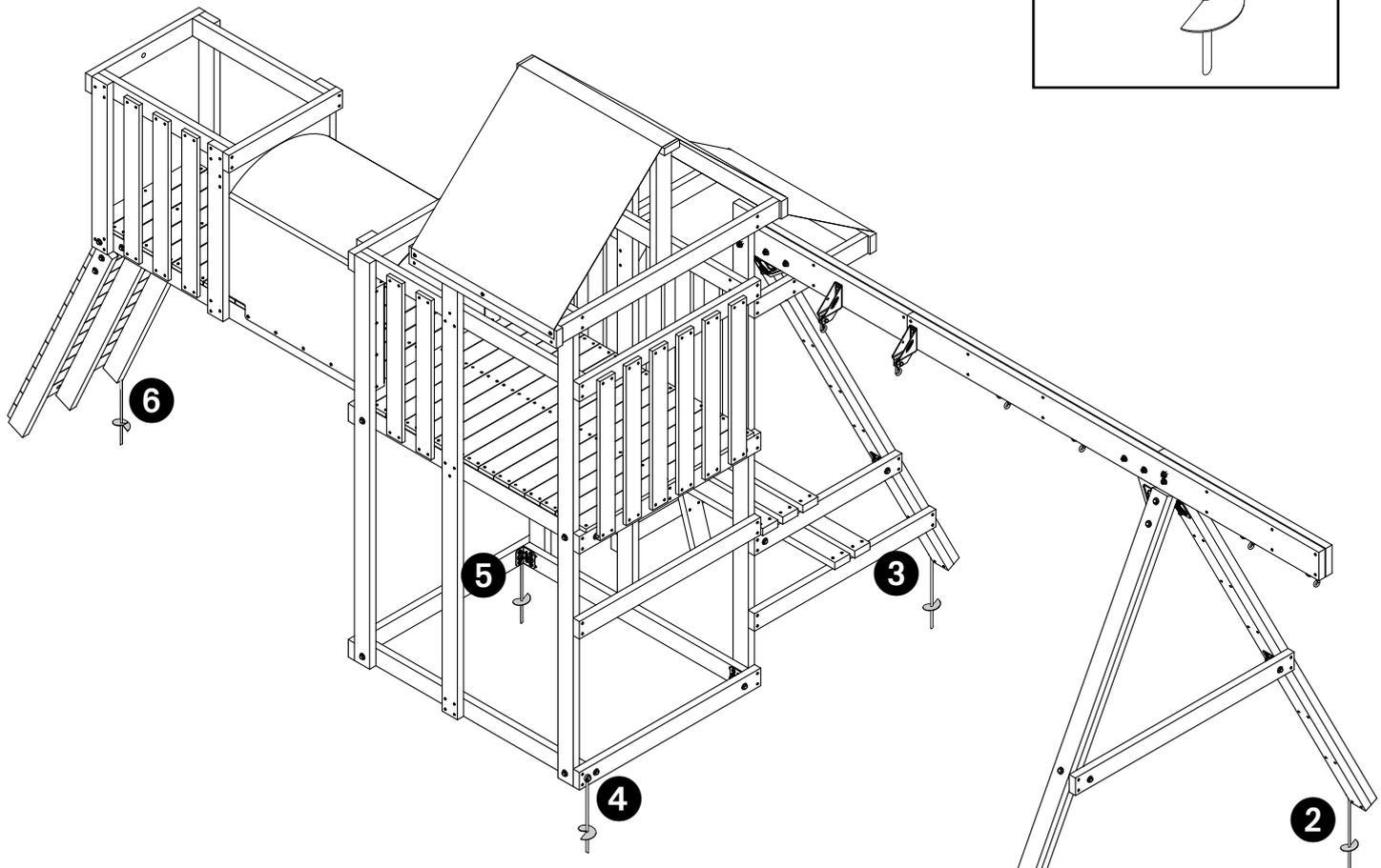
**Note:** If soil conditions permit anchors to be pulled out easily, such as in sandy soil conditions, cementing is required. If your ground is too hard to screw in the anchors you can remove the earth with a shovel. Install the anchors and compact the earth as you replace it. Anchors must be placed below the level of the shock-absorbing surfacing material to prevent tripping or injury resulting from a fall.
