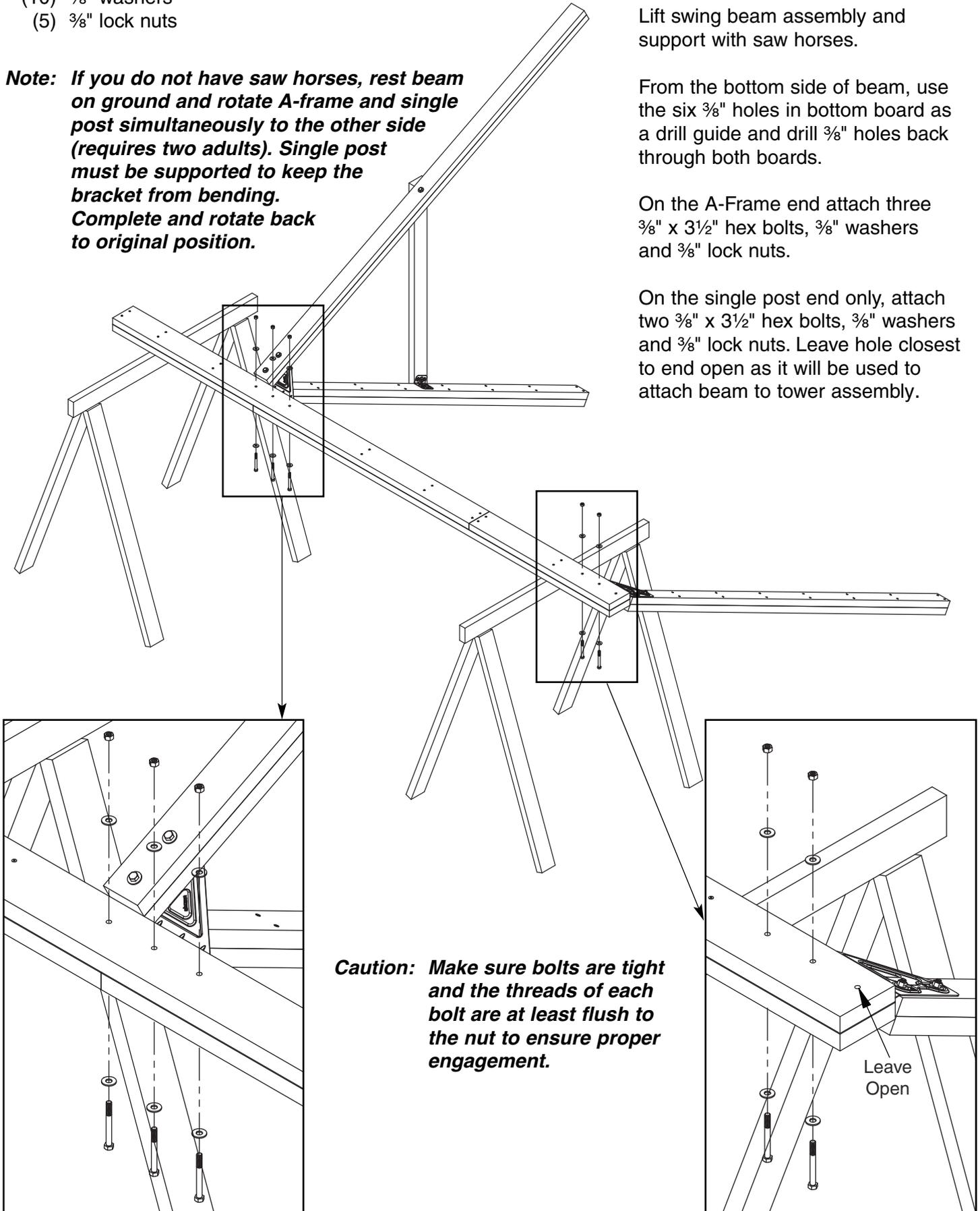
**Caution:** *Make sure bolts are tight and the threads of each bolt are at least flush to the nut to ensure proper engagement.*
